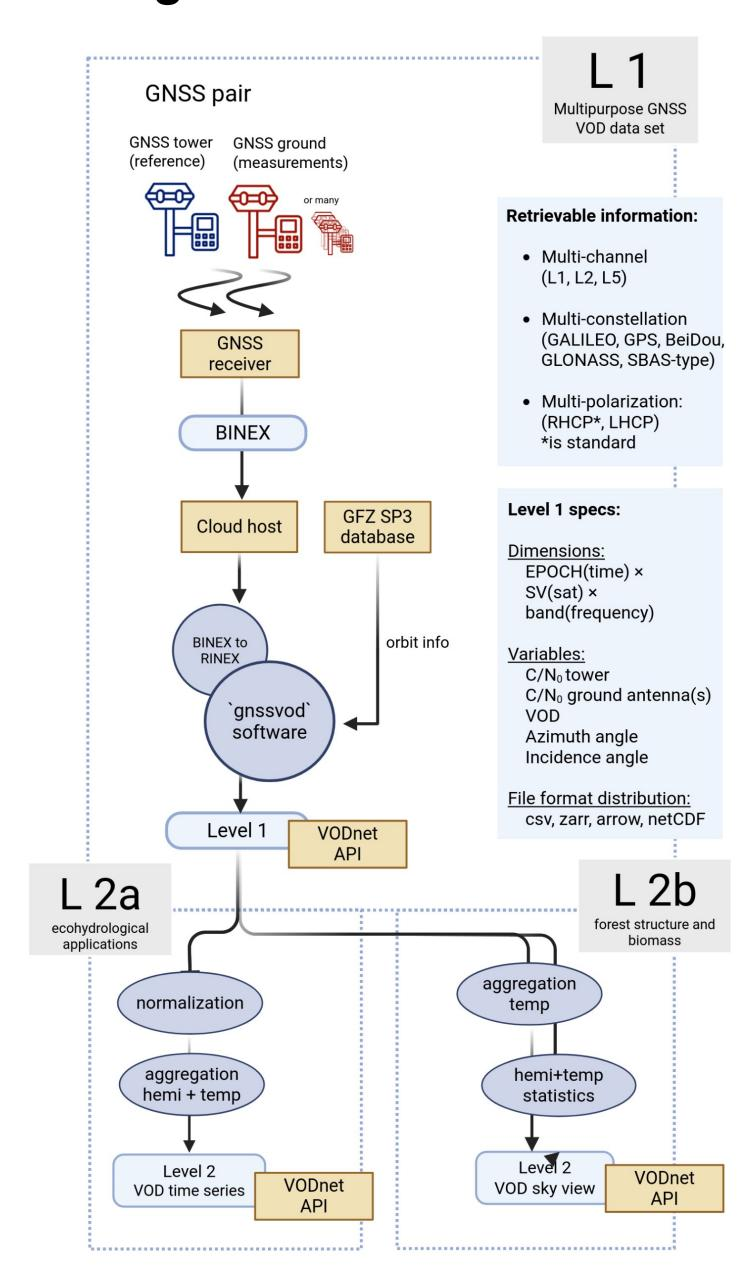
Based on the GNSSVOD python toolkit (Humphrey 2025), a common data pipeline for the various partners' setups will be developed, incl. readers accounting for divers receiver hardware.
